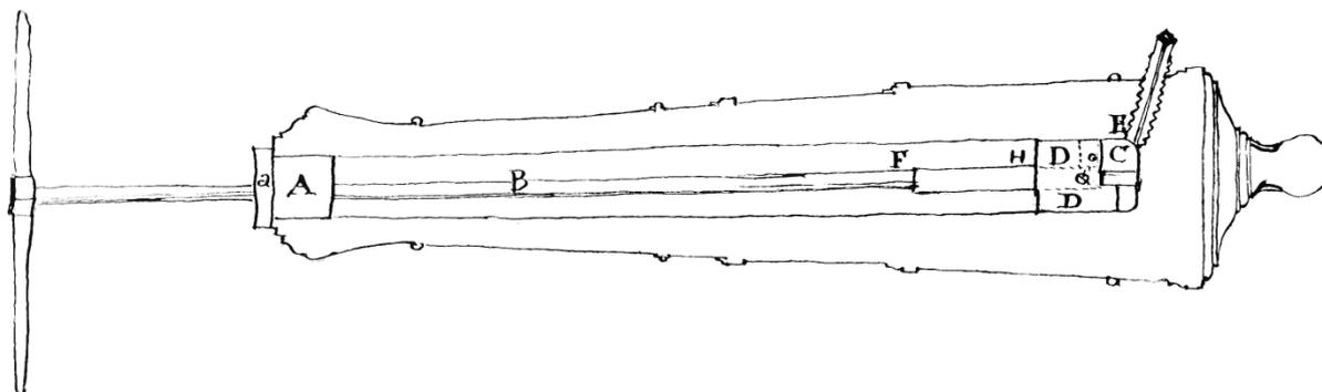
**Instrument for cutting off the copper vent-screw associated with the Verbruggens give an indication of the construction of the secret tool used by the same to repair the bore of guns.**
